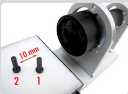
Images of two identical screws. Screw "1" is 10 mm closer to the lens. As you can see with telecentric lenses object size remains the same.
