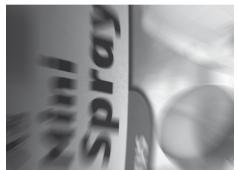
Without tilt adjustment the object is not homogeneously focused
