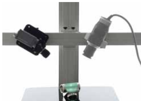
MCSM1-0.1x combined with a Scheimpflug projector at 90°
