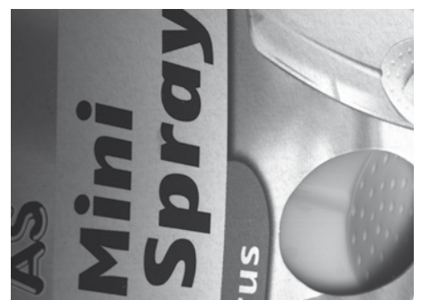
At the Scheimpflug angle the entire image becomes sharp
